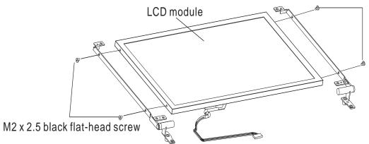
Figure 4-20 Removing the LCD module and screws
